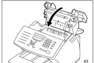
Press down on the Top Cover until a "Click" is heard to ensure the latches engage.
